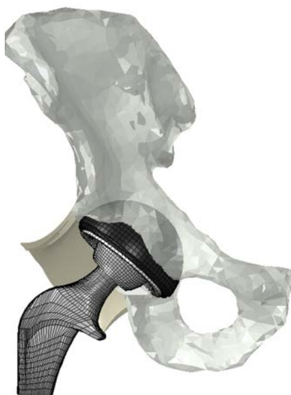
Figure 11: The capsule FE model of THA. The model consisted of THA hardware, bony anatomy and the hip capsule.
